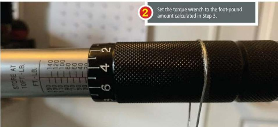
**2** Set the torque wrench to the foot-pound amount calculated in Step 3.
